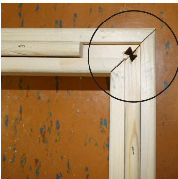
Fig. 2: Connect the floor frame elements
